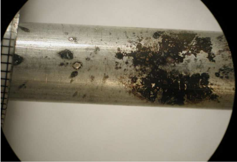
Figure 7: Test 9 - Slight damage to the aluminum tube
