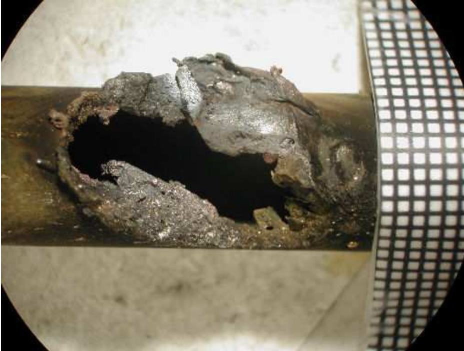
Figure 3: Test 23 Damage to Aluminum Tube.
