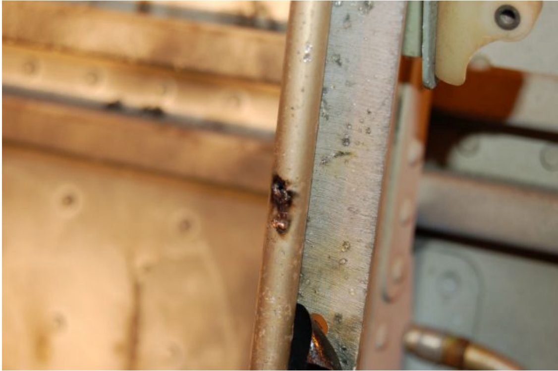
Figure 19. Post Test photo of damage to the aluminum hydraulic line.
