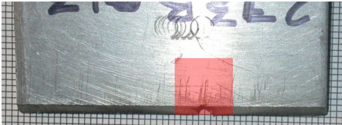
Figure 17. Comparison of actual blade damage to theoretical damage (red square) if all the arc energy was used to melt the aluminum blade.
